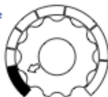
Figure 2: Pulsating pressure for cleaning zone
